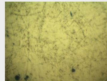
Cracks in case precoat is too brittle.
